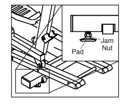
turn the leveling pads as needed until the elliptical crosstrainer is level. When the leveling pads are properly adjusted, firmly retighten the jam nuts.
